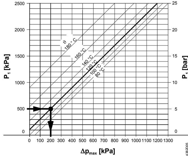
$\Delta p_{\max}$  = Differential pressure with valve almost closed, at which cavitation can largely be avoided
