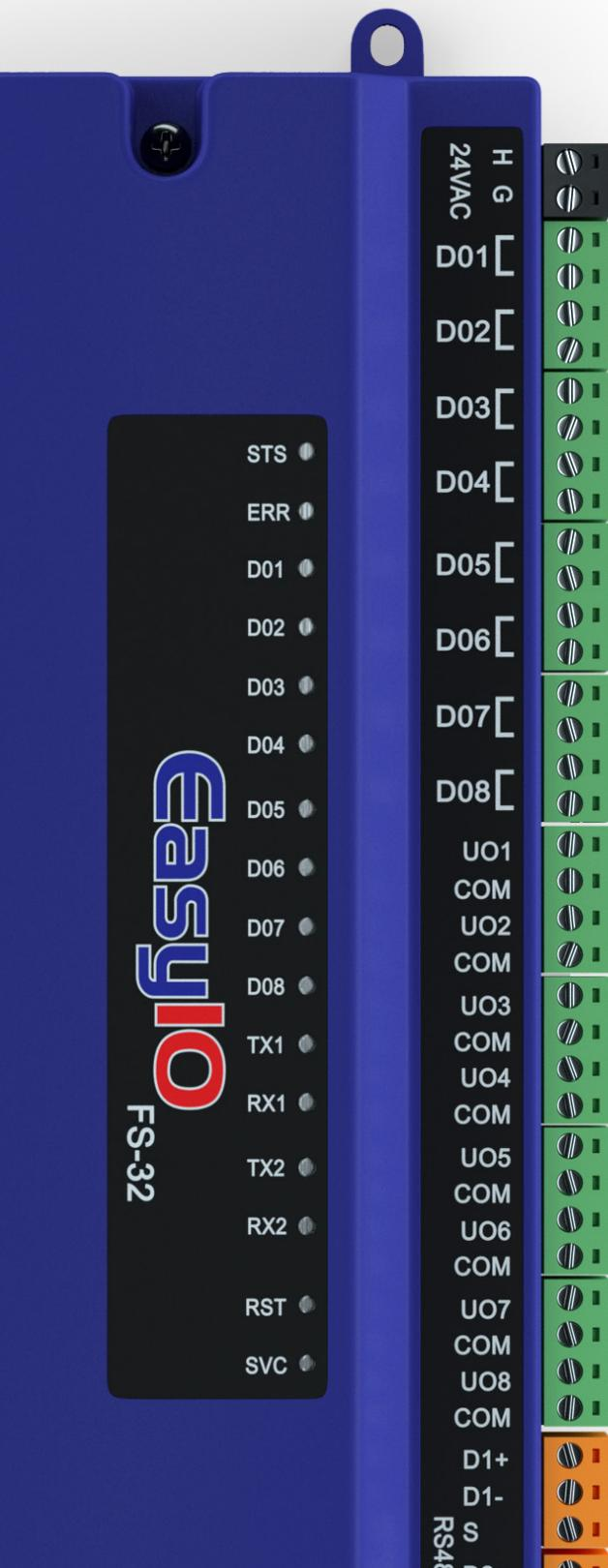
The FS-32 is a high-performance server class controller with a 1.2 GHz quad core processor, 512 MB RAM and 8GB flash memory, powerful capabilities with HTML5 graphics and multifunctional adapter widgets. The built-in VPN client/server allows for secure remote connectivity in line with your client's corporate policy, a unique feature for BMS controllers. The FS-32 supports IT standards, such as IPv6, 802.1x, MQTT publish/subscribe and REST API.
